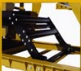
Bottom Bale Control Arm gently lowers the bale without causing damage
